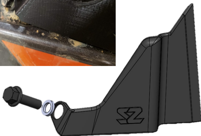
9. Install the front filler panel with the front filler panel shims inside the hole as shown above. These act as a crush sleeve for the plastic panel
